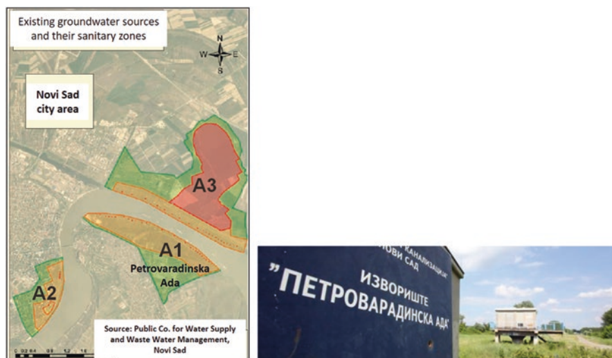
Fig. 23.4 Existing groundwater sources in Novi Sad with sanitary protection zones and Renney well at Petrovaradinska Ada groundwater pond (A1)
